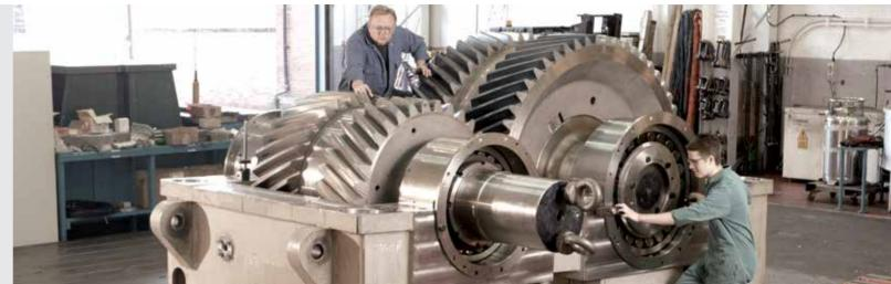
David Brown has extensive experience in the design and manufacture of primary drives for pinion stands, for both hot and cold rolling mills, and for new and existing applications. David Brown can offer total design flexibility to tailor the gearbox to the application, offering powers up to 15MW and torques up to 2.5 MNm. With gearboxes weighing up to 250 tonnes, David Brown are also able to advise and assist with site installation and commissioning.
